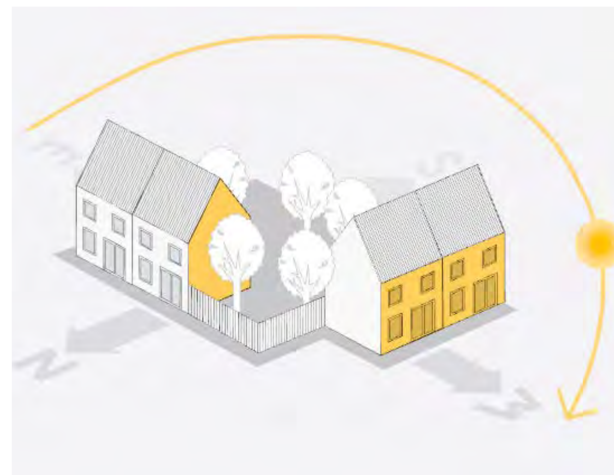
Figure 317: South easterly orientation maximises early morning solar gains and reduces overheating in the afternoon
